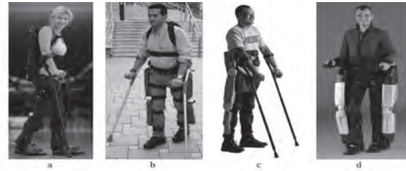
Figure 2. Mobile medical exoskeletons. (a) Ekso, (b) ReWalk, (c) Indego, (d) REX.
