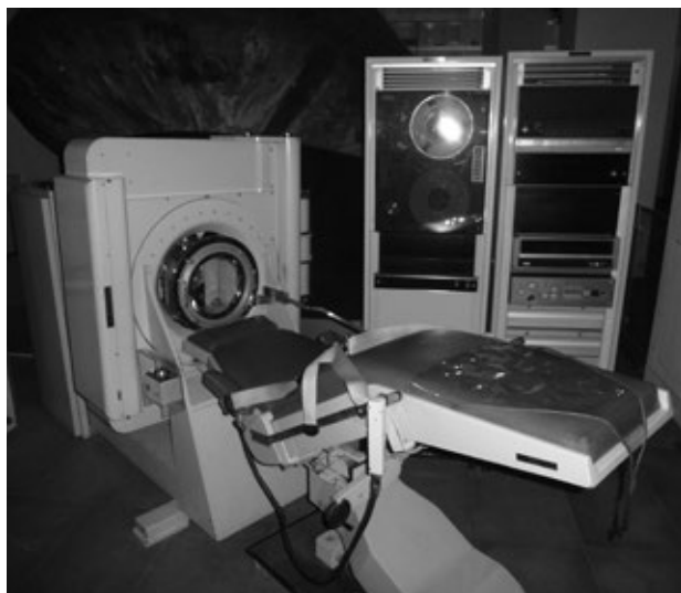
Figure 7. The first EMIICT scanner from Atkinson Morley's Hospital on display in the Science Museum, London.
